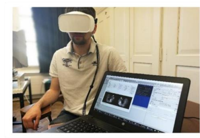
Fig. 3 Experimental VR set-up. The device is multi-functional (8 examinations in one device), mobile, suitable for bedside testing, and patient-friendly, generating objective, reproducible and quantifiable results. The examination is time-efficient and well tolerated. The optical stimuli are presented. Real-time registration of eye movements on notebook. Source: Private source, machineMD
