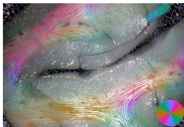
Fig.: Identification of fibre tracts using Mueller polarimetry in reflection configuration, color-coded for spatial orientation.
